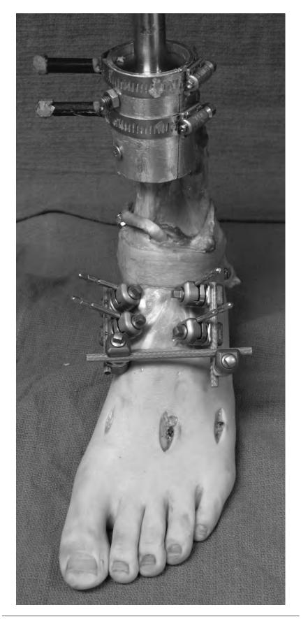
Figure 1: Stryker pins in the medial and lateral talus and navicular with Stryker external fixation hardware attached, including six clamps and three rods. The clamps were tightened to simulate fusion.
