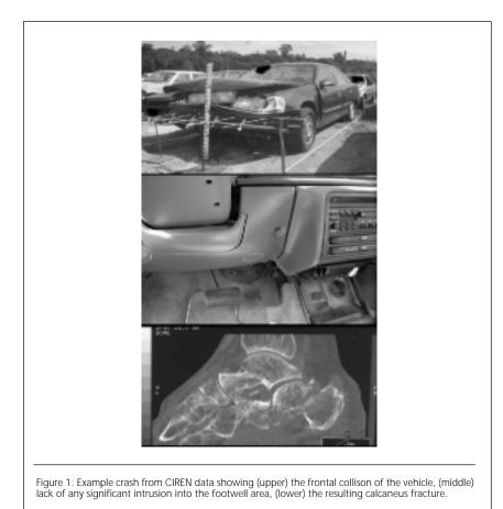
crushed floorpan may be causing foot injuries. These observations, along with epidemiological data, demonstrate that the brake pedal, specifically how it aligns the foot during a frontal collision with the driver braking, is a source of foot injuries. New technologies, such as "drive by wire", that is without mechanical linkages, will allow placement of driving controls, including the brake pedal, in positions which could reduce the potential for foot injury.
